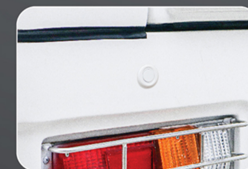
Rear Parking Sensors
